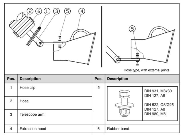
Proceed as follows for the installation of the extraction hood to the telescope arm:
